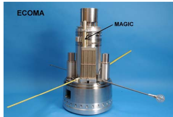
Part of the German-Norwegian ECOMA payload, carrying two MAGIC particle instruments (arrow) in combination with experiments addressing charged particles as well as neutral and ionospheric properties of the background atmosphere.
