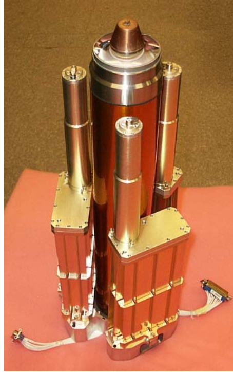
The instrument package for the MAGIC rocket flight consisting of MISU's hygrometer (center) and three NRL MAGIC particle samplers. The MAGIC campaign is scheduled at Esrange, Sweden, in January 2005.
